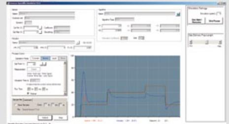
After performing an integrated system calibration and identification procedure, the auto-tuner instantly generates the optimum controller parameters for your process by using advanced inverse dynamics algorithms to analyse the collected data.
