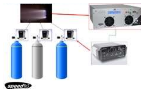
Figure 2: Adding a Speedflo Mini to the system allows the control of three different gases, which increases to eight gases with Speedflo standard.
