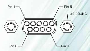
\* Connection to +15V OPEN, Connection to -15V: CLOSE (Normally closed valve model) Connection to +15V CLOSE, Connection to -15V: OPEN (Normally open valve model)
